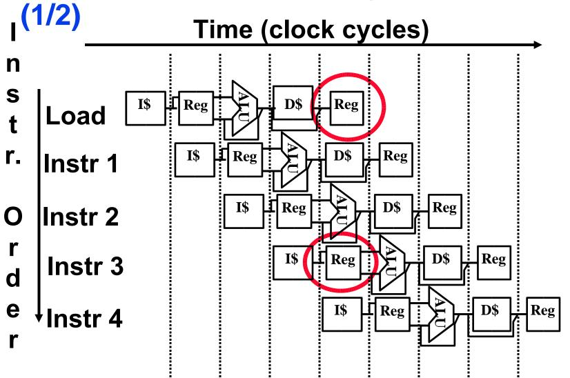
Can't read and write to registers simultaneously
