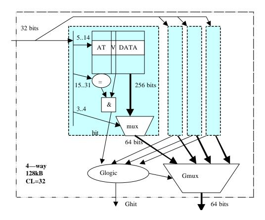
The four identical blocks each produces two identical signals: hit and data, numbered from left to right: hit 0,1,2,3 and data 0,1,2,3. At most one of the hit signals will be asserted at any one time. The new Gmux selects is controlled by the four hit signals and selects the data corresponding to the block with its hit signal asserted. The Ghit signal is the or function of the four hit signals. (Note the new bit range on the index, mux select and comparator fields in each block)
