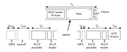
Fig. 1. Successful transmission of a single frame
