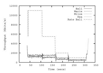
Fig. 10. Measured throughput in Mb/s for four hosts, UDP traffic
