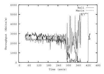
Fig. 11. Measured throughput in Mb/s for two hosts (one mobile), TCP traffic
