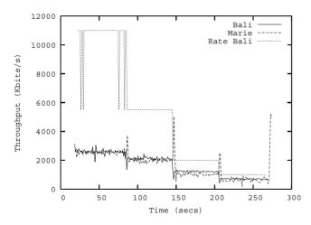
Fig. 5. Measured throughput in Mb/s for two hosts, TCP traffic
