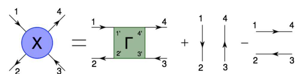
In the composition of the two-particle Green function, the susceptibility is the fully irreducible vertex part.
