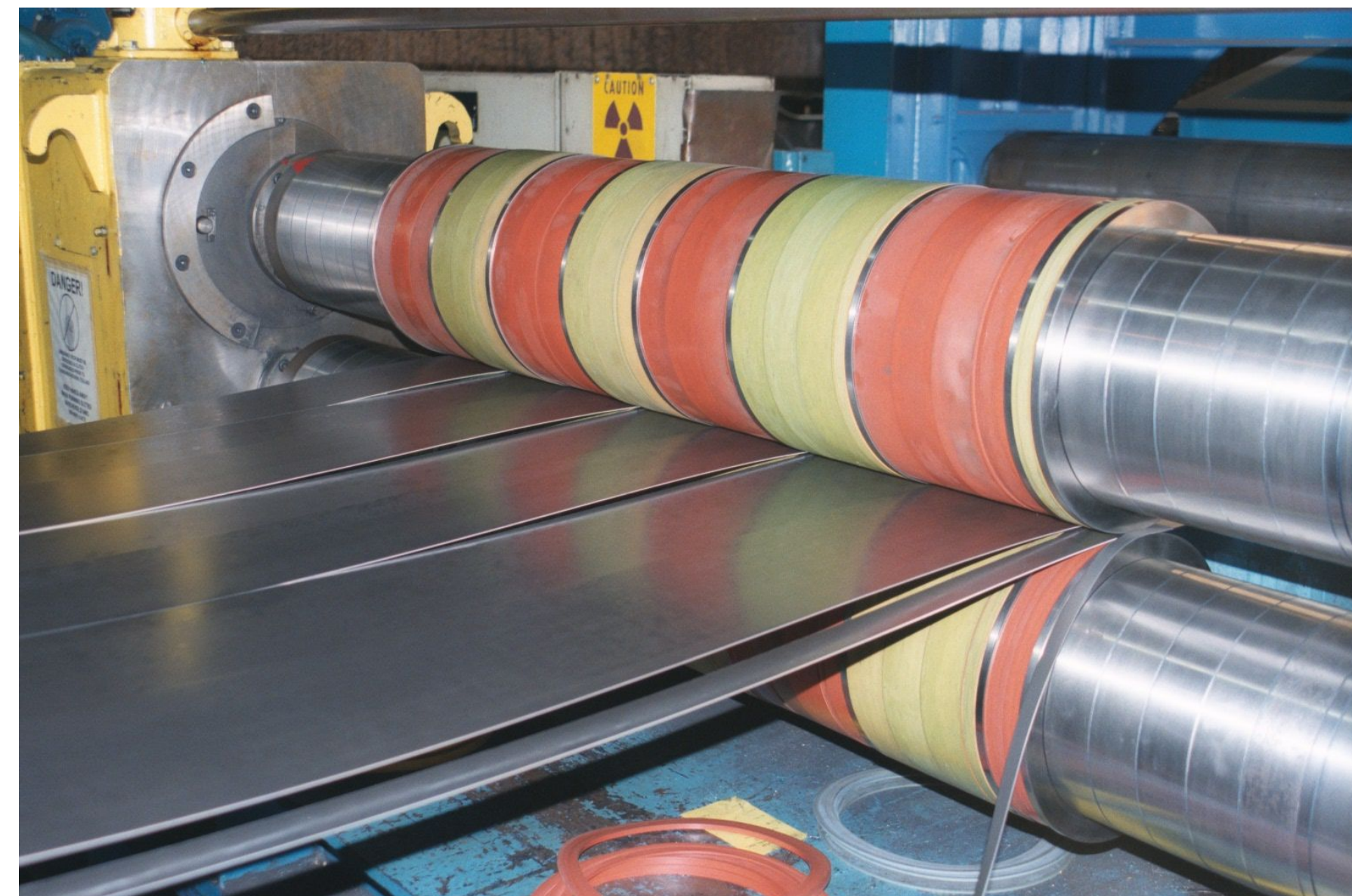
Figure 1: Example of industrial steel slitting, closely mimicking the setup at SSAB.
