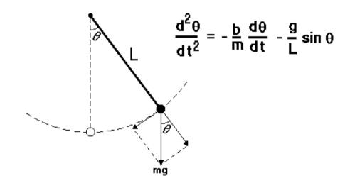
θ is the angle the pendulum has moved from the vertical, **L** is the length of the pendulum, **g** is the acceleration due to gravity, **m** is the mass of the pendulum, and **b** is a damping coefficient.
