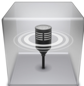
Figure 3.3: An intuitive illustration of an impulse response: a sound beep ripples an acoustic signal through a room.
