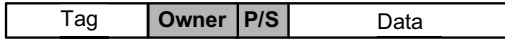
(a) Coupled LLC-directory implementation: LLC tags are extended to hold private/shared classification. The owner field is valid when a cache line is classified as private.
