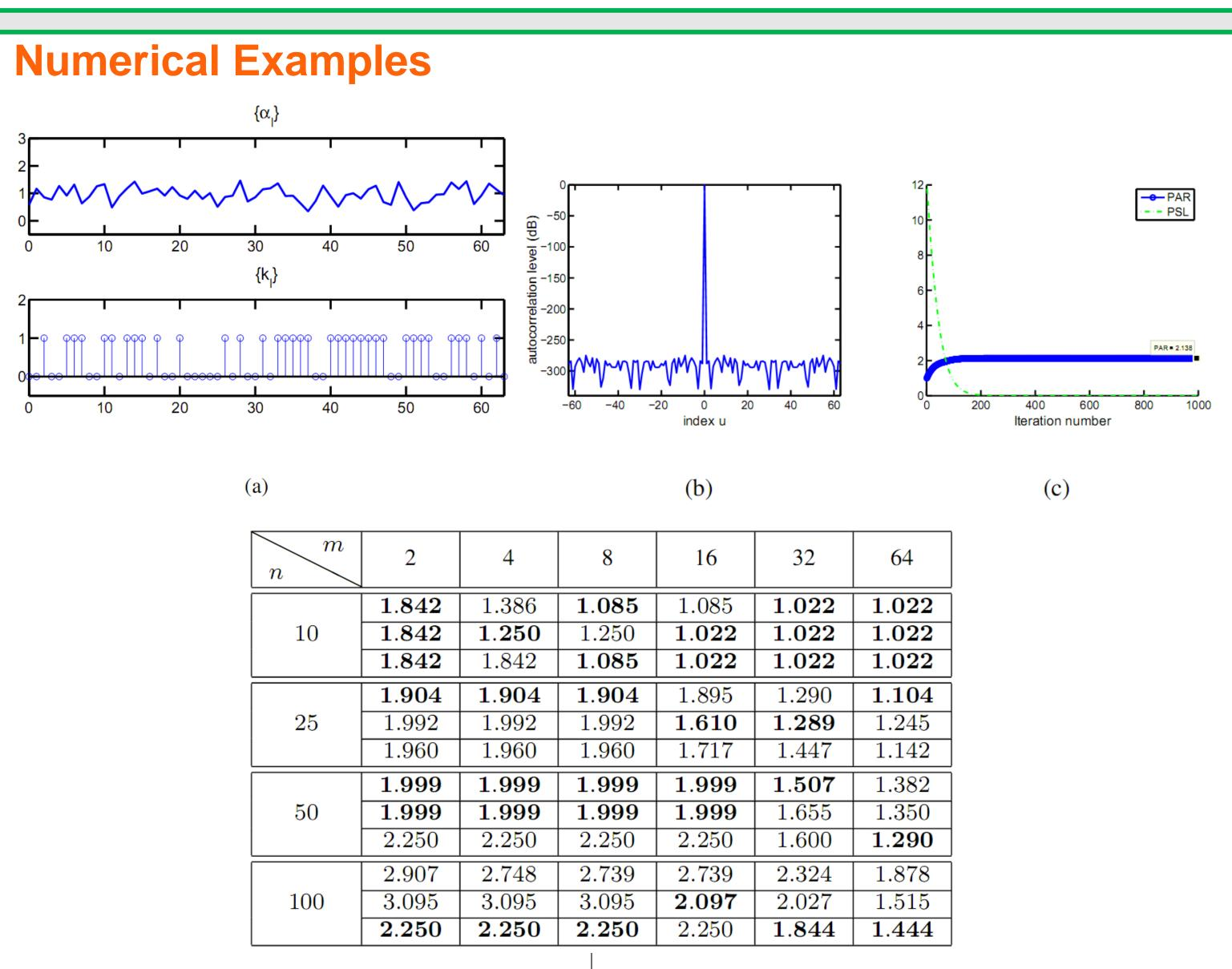
**Fig. 1**. Design of a phase-quantized sequence of length n=64 with low PAR via the alternating projection method. The phase quantization level is m=2. (a) the sequence amplitudes  $\{\alpha_l\}$  and integer phases  $\{k_l\}$ . (b) the autocorrelation levels (in dB) of the obtained sequence. (c) the PSL and PAR vs. the iteration number for the obtained sequence. The sequence achieves practically perfect periodic correlation properties and PAR = 2.138.
