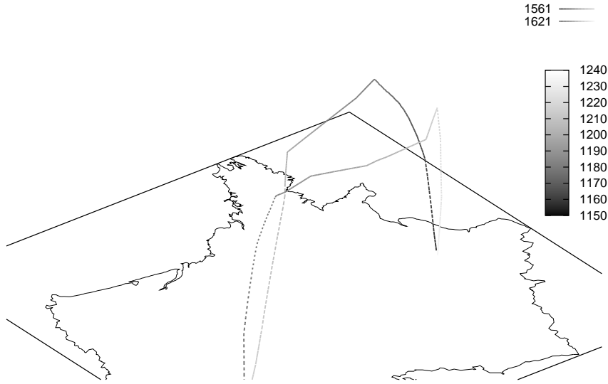
Figure 4 Three potential conflicts between two flights: one near Paris airport at low altitude and two other en-route at the cruising altitude of the lower flight. The gray scale corresponds to time (in minutes) along the trajectory, the lighter the later.
