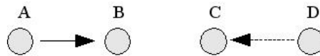
Figure 3.5: In this situation, D to A transmission will have half the bandwidth of the network
