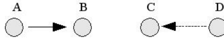
Figure 3.9: In PAMAS, nodes can answer to a RTS by the control channel
