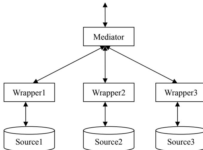
Figure 2-2: The mediator/wrapper architecture
