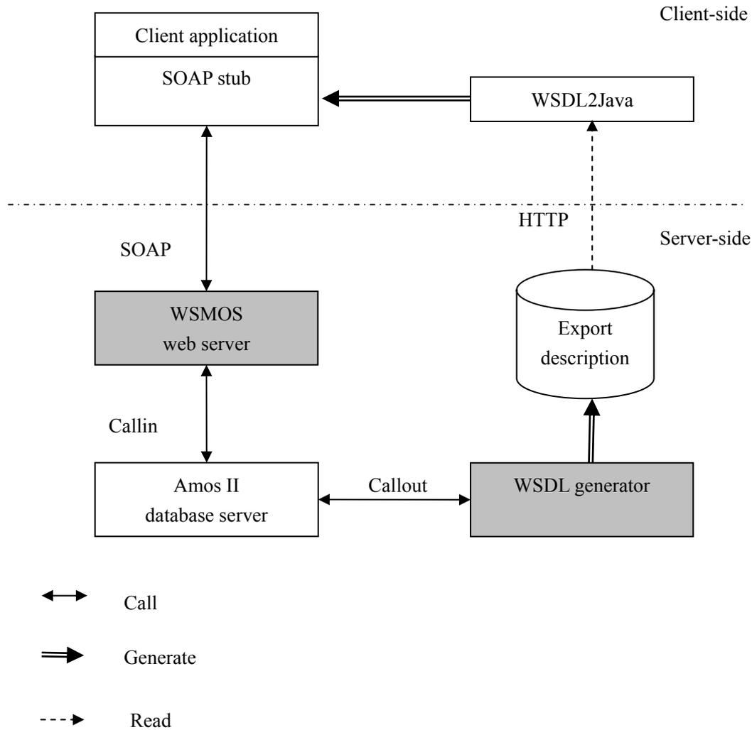
Figure 6-1: The architecture of WSMOS
