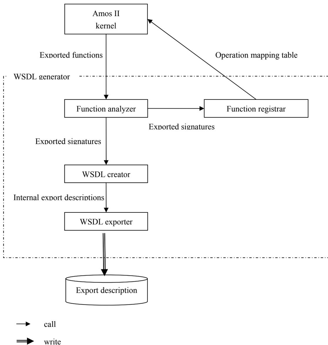
Figure 6-2: WSDL Generator modules
