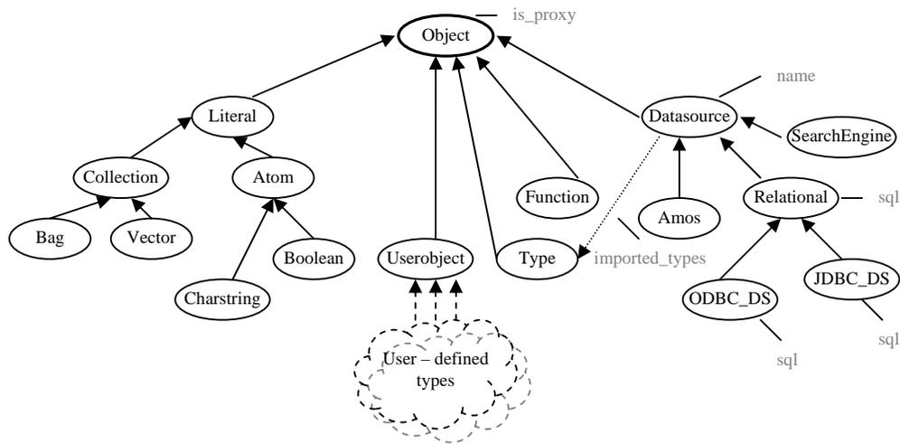
Figure 2.3: AMOS II system type hierarchy [8]
