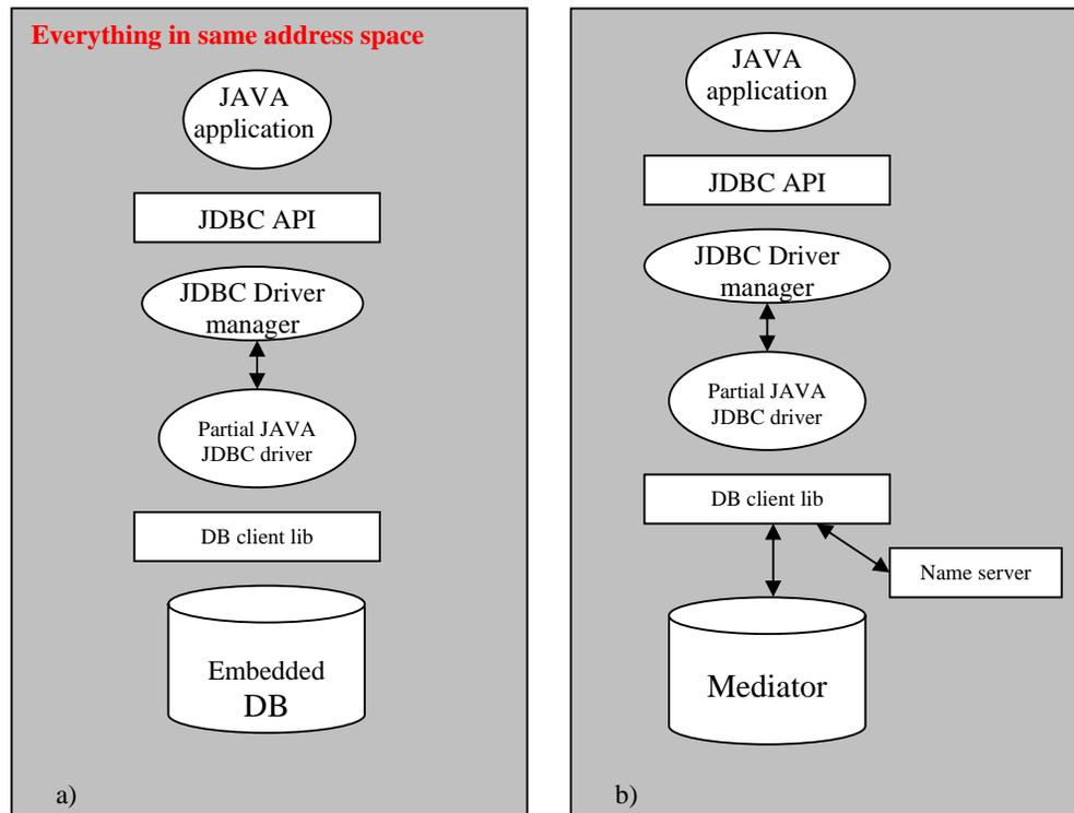
Figure 4.2: Chosen driver architecture: a) Connected to embedded database b) Connected to mediator peer with help of name server
