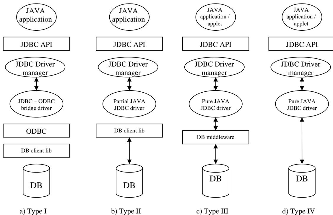
Figure 4.1: Four classical types of JDBC driver architecture
