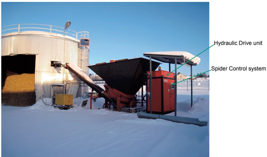
Figure 5. A wood waste shredder at Mellansel plant
