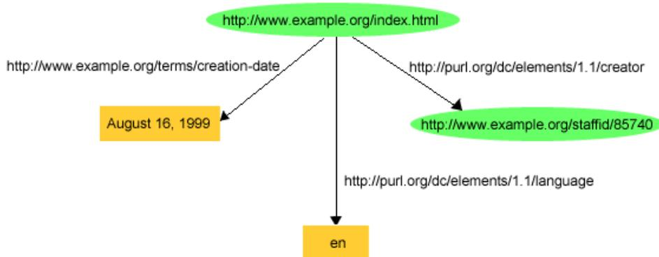
Figure 5 A RDF graph to explain triple notation
