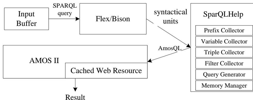
Figure 10 Architecture of SparQL Parser
