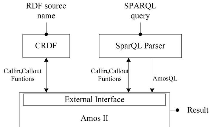
Figure 8 Architecture of SPARAMOS
