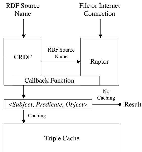
Figure 9 Architecture of CRDF
