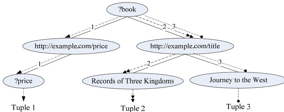
Figure 12 Example of Triple Pattern Tree
