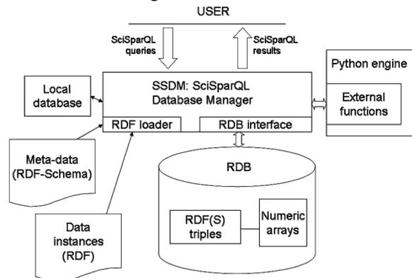
Fig. 1 Overview of SSDM architecture
