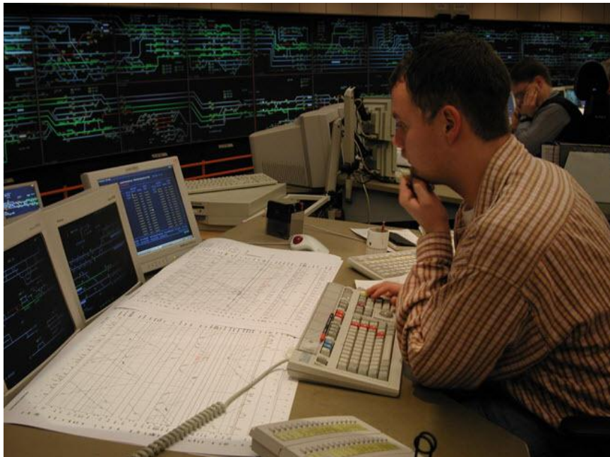
Figure 2. The picture shows the work place of a traffic controller today at the train traffic control centre in Stockholm, Sweden. The picture shows large wall panels, smaller computer screens as well as a paper-based time-distance graph.
