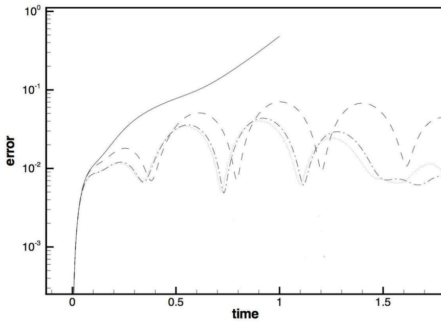
Figure 3: Time history of  $l_2$  error for 4 different values of penalty strength  $\gamma$  for the standing wave simulation with coarsest triply-periodic unstructured grid. *solidline*:  $\gamma = 0.99$ ; *dashedline*:  $\gamma = 1$ ; *dashed – dottedline*:  $\gamma = 1.2$ ; *dottedline*:  $\gamma = 5$
