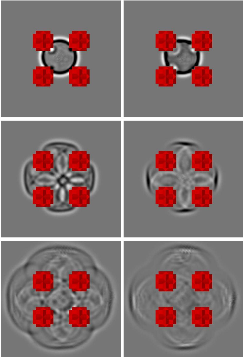
Figure 6: Propagation of a 3D Gaussian pulse comparing Neumann (left column) and Dirichlet (right column) boundary conditions (for three times,  $t = 0.25$ ,  $t = 0.5$ , and  $t = 0.75$ ) on the  $2 \times 2 \times 2$  array of 3-cube compounds.
