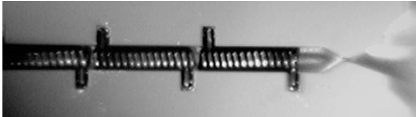
Figure 1: A micro machined nozzle with three heater coils positioned just before the nozzle throat. The nozzle throat is approximately 30\mu\text{m} in a heat exchange chamber.
