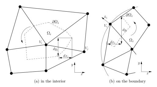
Figure 1: The grid (solid lines) and the dual grid (dashed lines).
