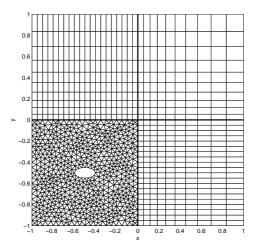
Figure 9: A hybrid mesh with four sub-domains.
