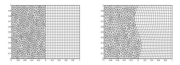
(a) with a linear interface. 702 nodes are used on (b) with a curved interface. 597 nodes are used on the left domain and  $21 \times 21$  nodes are used on the the left domain and  $21 \times 21$  nodes are used on the right domain.
