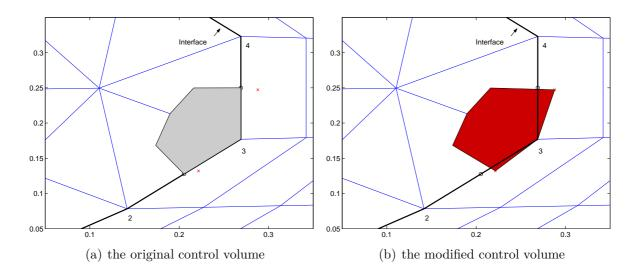
Figure 4: The control volume connected to point 3 at the interface.
