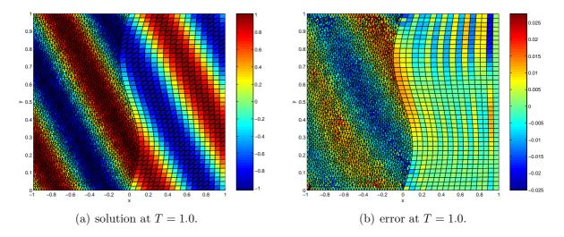
Figure 8:  $\log_{10}(L_2 - error) = -2.22$  on the left subdomain with 2302 nodes and  $\log_{10}(L_2 - error) = -2.39$  with 738 nodes for  $u_t + u_x + u_y = 0.1(u_{xx} + u_{yy})$ . A curved interface is used.
