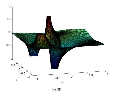
Figure 11: The temperature distribution around four rods.
