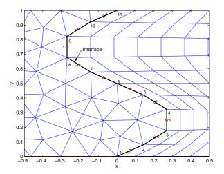
Figure 3: The black 'o' represents the midpoints of the interface and the red 'x' represents the new modified dual grid points.
