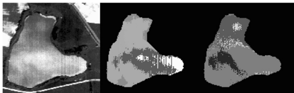
FIGURE: A very turbid lake (left) and the segmentation of watermasses by unsupervised classification (middle) and by thresholding the hue component of a IHS transformation of the three first principal components (right).
