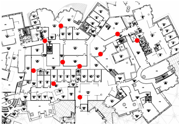
Figure 7—Node locations for one floor of the testbed.
