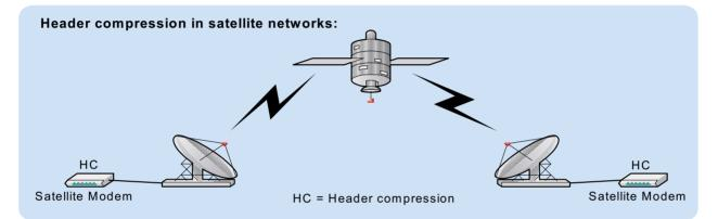
Satellite links have high bit error rates and high delays (delay varies from more than 500 milliseconds (ms) for geo-synchronous to a few ms for lower earth orbit satellites). The header compression module is part of satellite modem as shown above.
