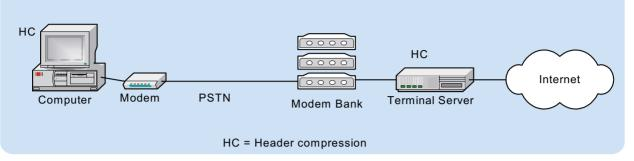
Internet access often uses modems and PSTN links, which have low bandwidth. To improve performance for interactive applications like Telnet, web services as well as Voice over IP, usage of header compression results in bandwidth savings. The header compression module is a part of the end user's computer operating system and the Terminal Server (PPP link end points) as shown in the diagram above.
