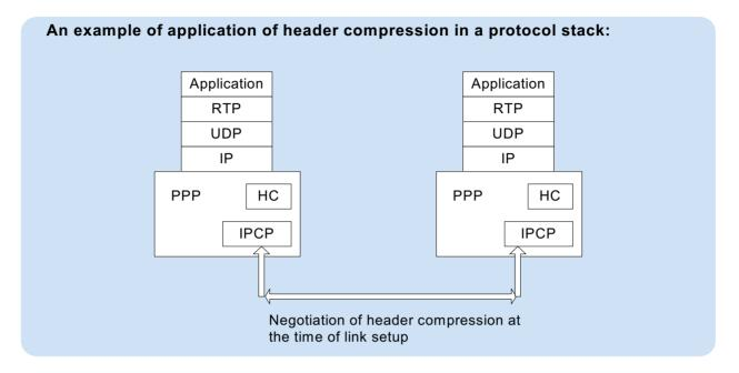
The above diagram shows the location of the header compression module in a protocol stack. The link layer for example PPP, uses the IPCP protocol to negotiate the use of header compression and related parameters at the time of the link set-up.
