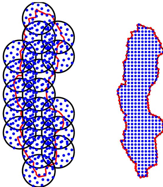
Figure 2: Illustration of RBF-PUM setup used to solve PDE for a computational domain shaped as continental Sweden. Left figure illustrates the patch cover and the right figure shows the points where PDE is enforced.
