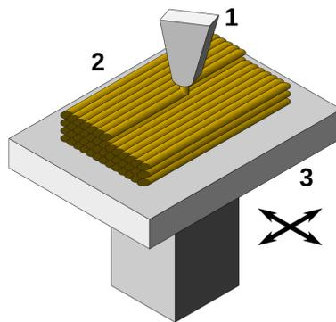
Figure 1: Illustration of fused filament fabrication (source: Wikipedia).
