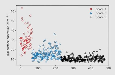
All passages were analyzed based on the classification using 3 scores. The result can be seen in the plot. The classes were separated by at least 75 %. Further, analyzing the spread of the passages made by the same cow within a certain class showed no clear clusters. Both results indicate that it is possible that the method can be used to compare rumen fill between different cows.
