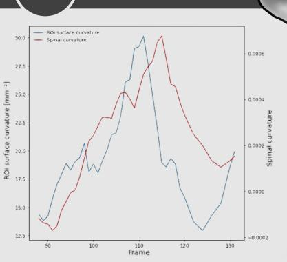
The walk cycle showed a high correlation between the spine curvature (red) and the ROI surface curvature (blue). It was concluded that the most reliable measurements were obtained when the spine was straight as can be seen in the figure above which is when spinal curvature is close to zero
