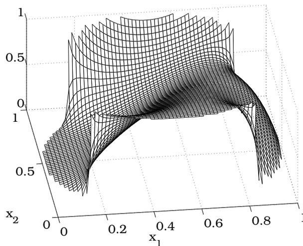
Figure 8.5: Solution of convection diffusion equation on an circular domain,  $\varepsilon = 0.1$ .
