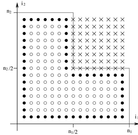
Figure 8.1: The L-shaped domain. Empty bullets denote grid-points in  $\Omega$ , filled bullets denote grid-points in  $\Gamma$ , and crosses denote irrelevant grid-points.
