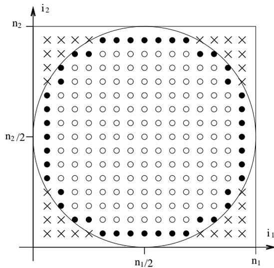
Figure 8.4: The circular domain. Empty bullets denote grid-points in  $\Omega$ , filled bullets denote grid-points in  $\Gamma$ , and crosses denote irrelevant grid-points.
