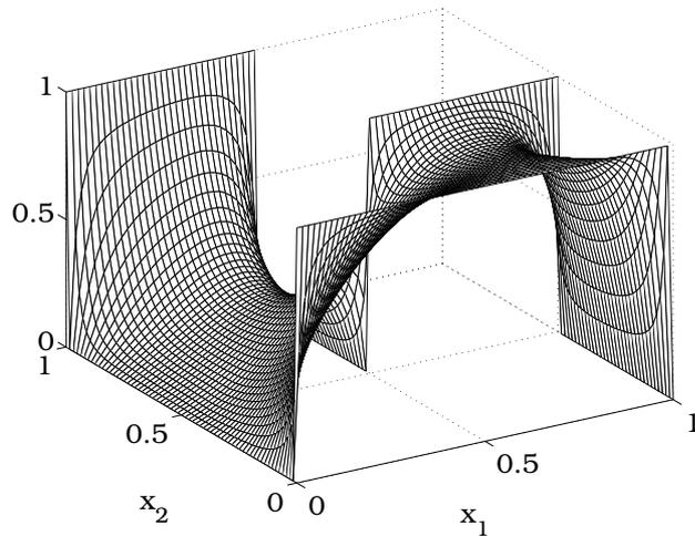
Figure 8.2: Solution of convection diffusion equation,  $\varepsilon = 0.1$  on an L-shaped domain.
