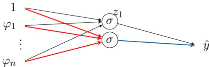
$$\begin{aligned} z_1 &= \sigma \left( \theta_{01}^{(1)} + \sum_{j=1}^n \theta_{j1}^{(1)} \varphi_j \right) & y &= \sum_{m=1}^2 \theta_m^{(2)} z_m \\ z_2 &= \sigma \left( \theta_{02}^{(1)} + \sum_{j=1}^n \theta_{j2}^{(1)} \varphi_j \right) \end{aligned}$$
